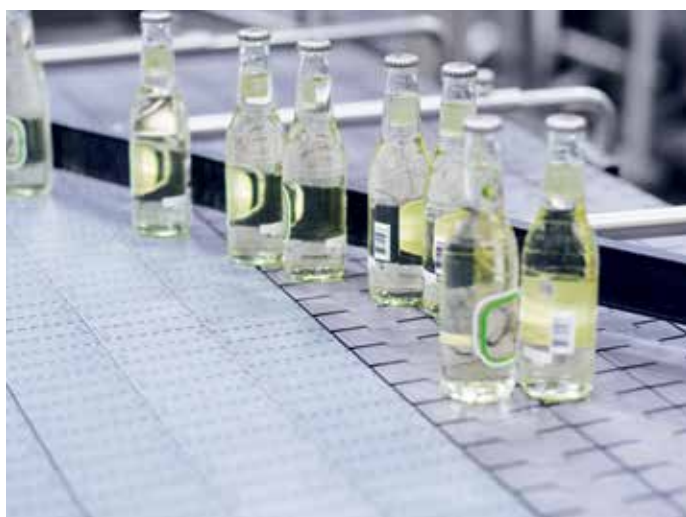
Bottles conveyor with FTDP1000 XLG MatTop® chain
