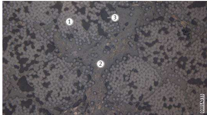
Figure 1 Microsection of the sliding layer of an ELGOTEX-WA filament wound bush
